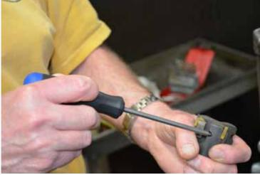
Factory preset torque level helps prevent damage to carbide inserts.
